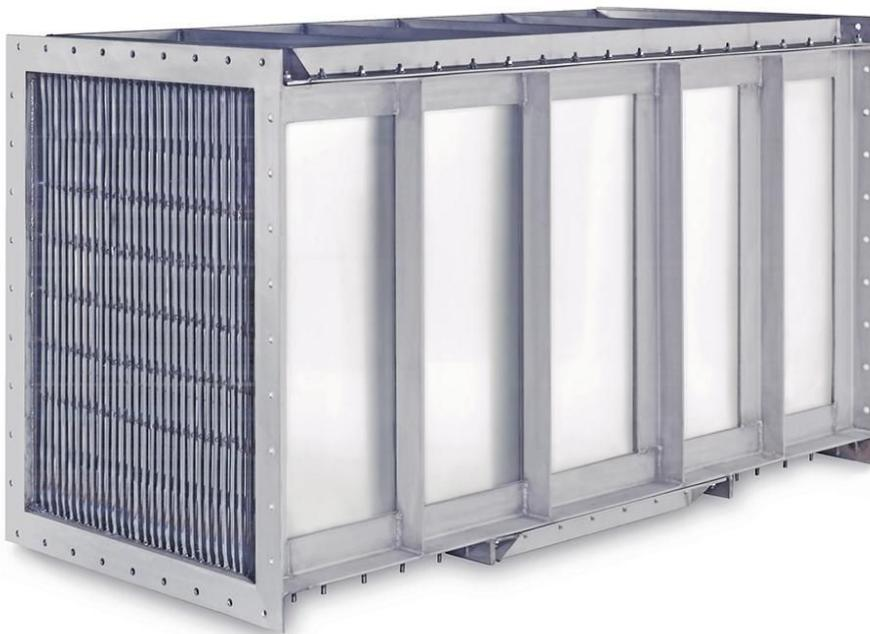
**FIGURE 3.** Plate-type heat exchangers use a series of nested plates to allow the exchange of heat between the two media without the two airstreams coming into contact with each other.
