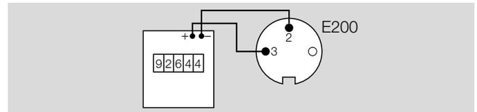
Electronic meter for digital remote indication of the current flow rate (in  $m^3/h$ ).
