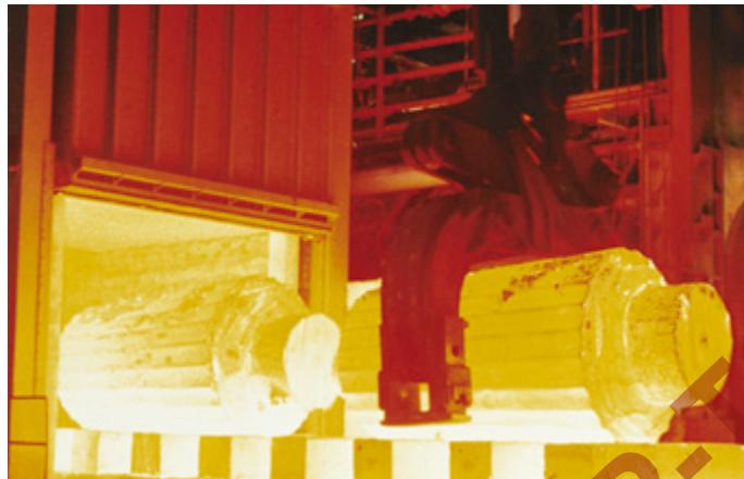
Metallurgical industry: forging furnace
