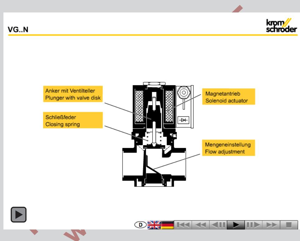
The interactive animation shows the function of the gas solenoid valve VG..N, quick opening.
