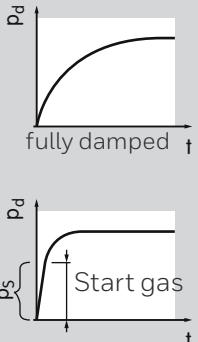
The gas solenoid valve VG..L opens within 10 s.
