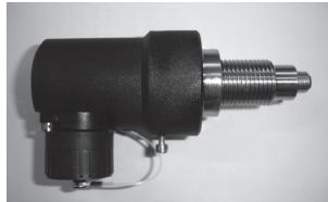
You can use **HF pulse generators** (Types A1R and A1S) for higher frequencies (if available). HF pulse generators are screwed into the meter housing pressure-tight. However, the connection plug can be turned.
