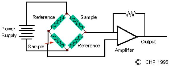
fig. 1-3 Typical electrical TCD circuit
