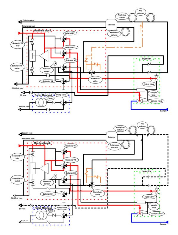
fig. 2-4 Internal Gas Flow Circuit for each Analytical Channel with backflush of the EnCal 3000, before activating backflush valve (top) and after activating backflush valve (below)
