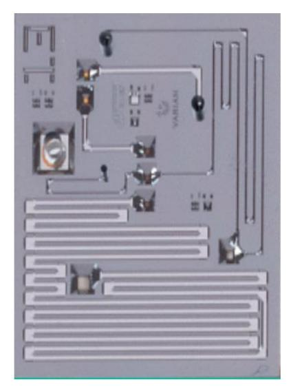
fig. 1-4 MEMS Sample Injector
