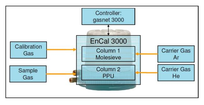
fig.2-16: Configuration with two Carrier Gases
