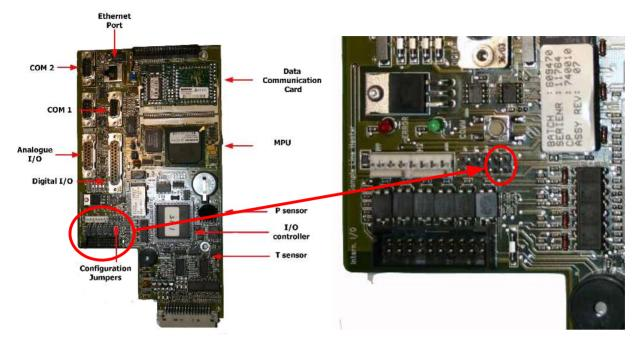
fig. 2-5 Save parameters in the measuring unit
