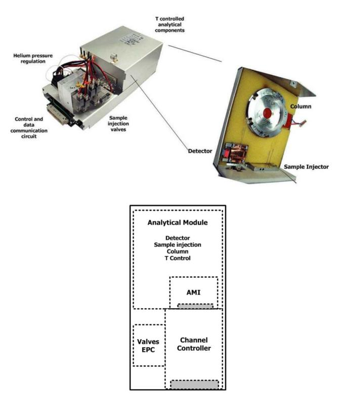
fig. 2-2 Overview of Channel Components
