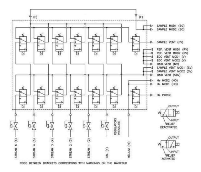
fig. 2-11 Flow diagram Sample Conditioning and Selection System
