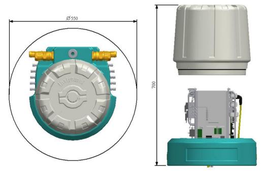
fig. 5-1 Mounting Dimensions and Installation Clearance
