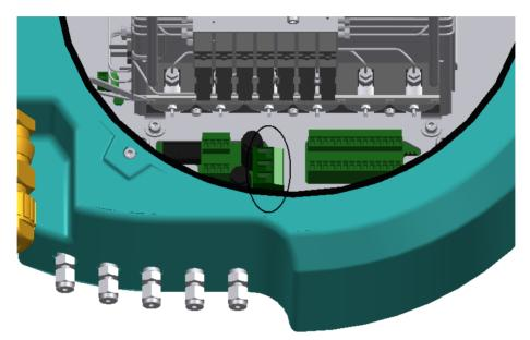
fig. 5-6 Location of Power Supply connector (J8)
