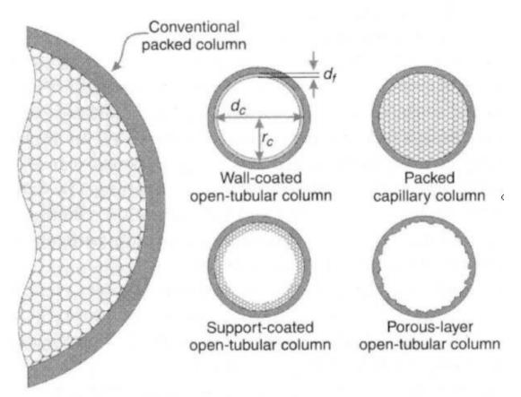
fig. 1-2 Different types of gas chromatographic columns
