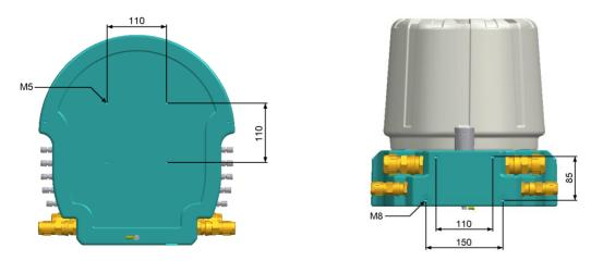
fig. 5-2 Mounting Holes EnCal 3000 Housing
