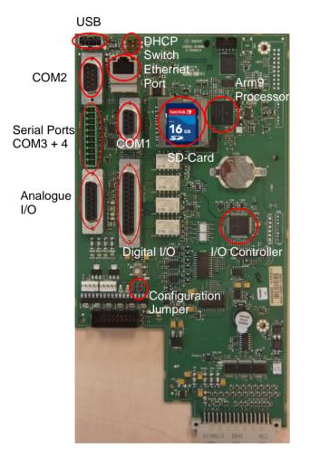
fig. 2-5: Processor Board connections
