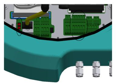
fig. 5-8 Location of Serial ModBus connector (J6)
