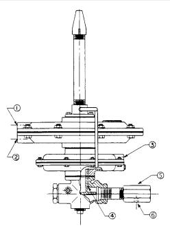
Figure 2. Cutaway of PCR
