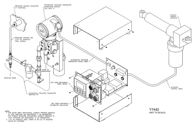
Figure 1. Dryer Pressure Control System Components
