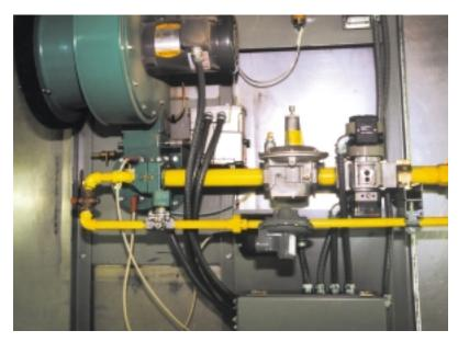
One of two Eclipse 200RM RatioMatic burners providing 10,000scfh of 400°F air for powder coating oven.
