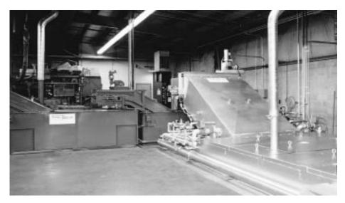
Eclipse Veri-Flame burner controls and other diagnostic components. A TBI semi-closed loop cooling system helps keep fans, hot pulley bearings, and cooling jackets cool utilizing a non-toxic coolant.
