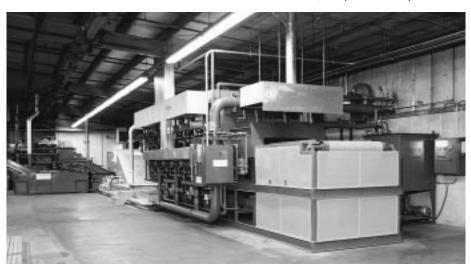
The austempering line at Eastern Metal Treating is a four-stage process. Parts are heat treated in 3-zone 1500° F hardening furnace, quenched to one desired hardness in a molten salt bath, desalinized in a cold water washer, and desalinized and rust treated in a final hot water washer.
