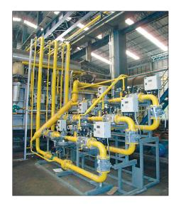
The gas control skids with safety shut off system, flow metering and flow control valves were designed and pre-assembled at Eclipse Suzhou PRC. The system was designed for operational ease and includes good access areas for maintenance.
