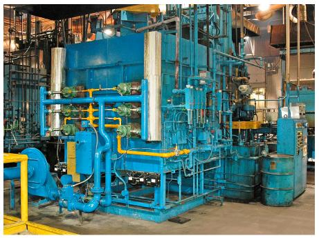
Back view of the furnace showing the location of the AutoRecupe burners.
