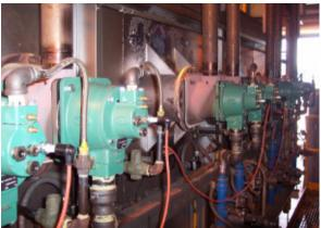
Close-up views of Eclipse AutoRecupe SER burners installed on multi-purpose metal treating furnace.
