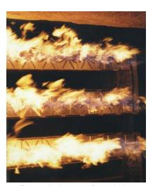
Burner being test fired during initial set-up.
