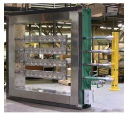
Packaged FlueFire Burner prior to installation
