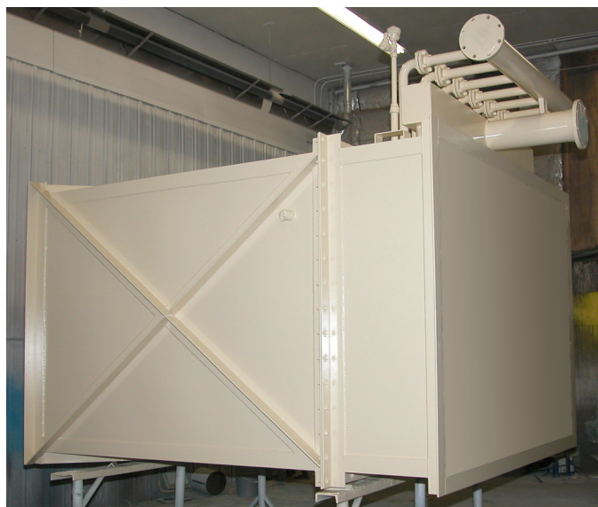
Pre-assembled duct section and combustion chamber simplify on-site installation.
