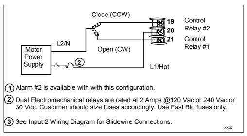
Figure 2-14 Position Proportional or Three Position Step Control
