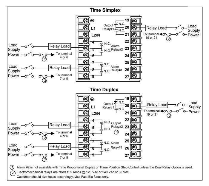
Figure 2-8 Electromechanical Relay Output
