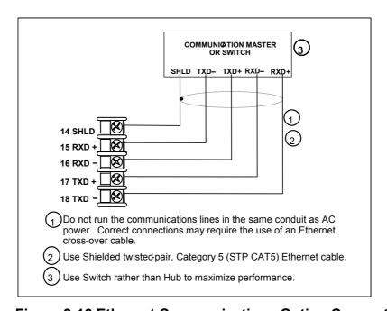
**Figure 2-16 Ethernet Communications Option Connections**
