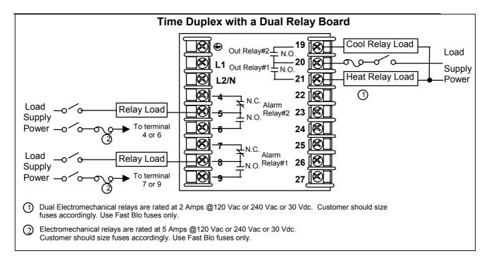
Figure 2-11 Dual Electromechanical Relay Option Output
