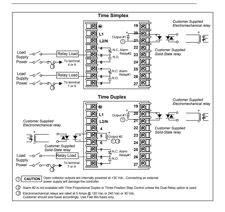
Figure 2-10 Open Collector Output
