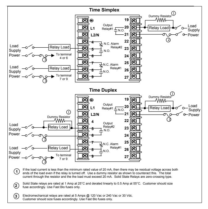
Figure 2-9 Solid State Relay Output
