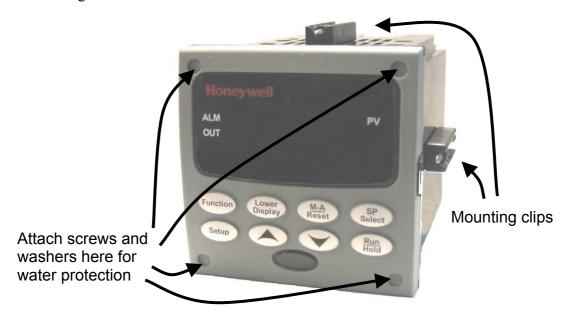
Figure 2-3 Mounting Methods
