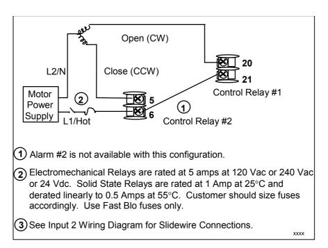
Figure 2-13 Position Proportional or Three Position Step Control
