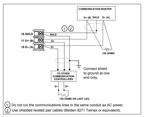
Figure 2-15 RS-422/485 Communications Option Connections
