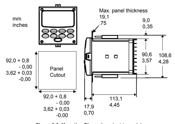
Figure 2-2 Mounting Dimensions (not to scale)
