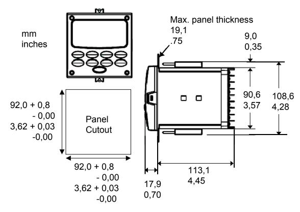
Figure 2-2 Mounting Dimensions (not to scale)
