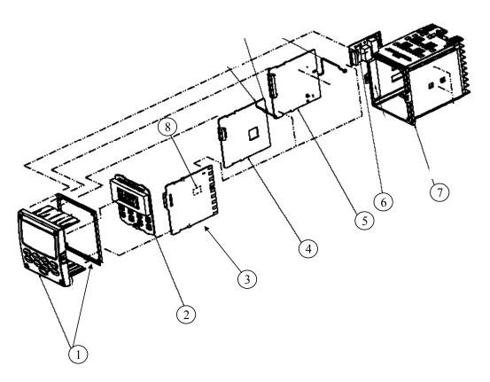
Figure 8-1 UDC2500 Exploded View
