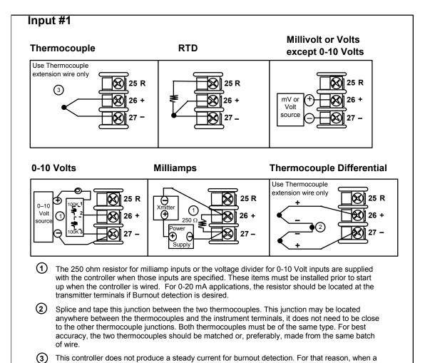
Figure 2-6 Input 1 Connections
