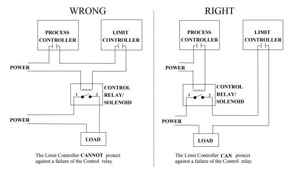
Figure 2-15 Limit Controller Application Diagram
