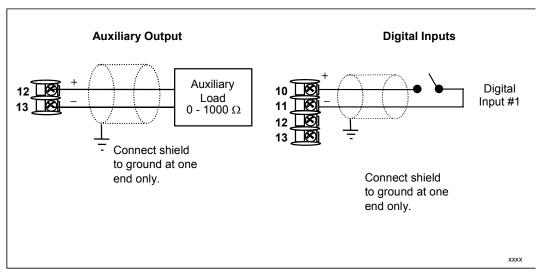
Figure 2-12 Auxiliary Output and Digital Inputs Option Connections
