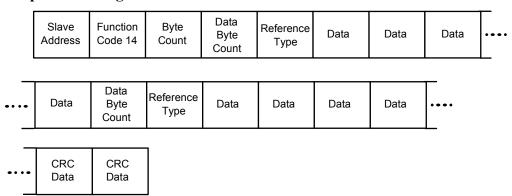
For Infrared Transactions, add three BOFs (C0hex) at the beginning of each message and one EOF (FFhex) at the end of each message.
