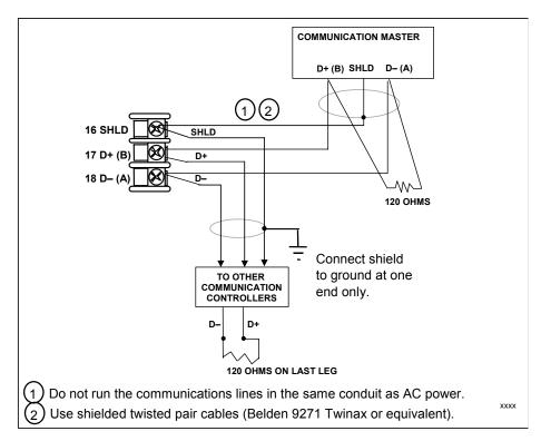
Figure 2-10 RS-422/485 Communications Option Connections
