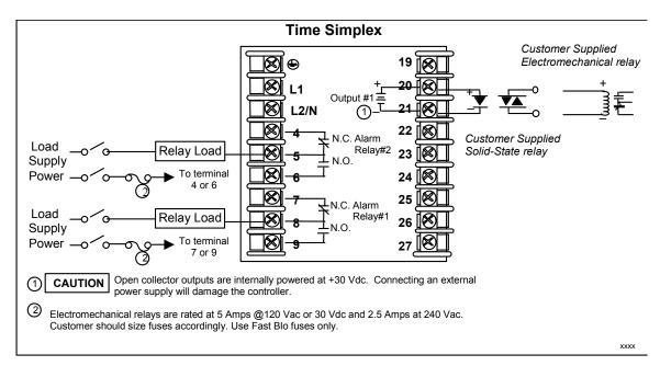
Figure 2-9 Open Collector Output
