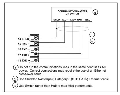
**Figure 2-11 Ethernet Communications Option Connections**
