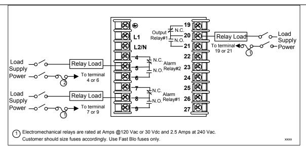
Figure 2-7 Electromechanical Relay Output
