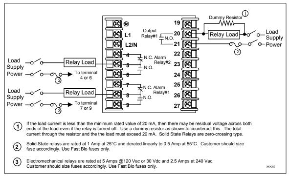
Figure 2-8 Solid State Relay Output
