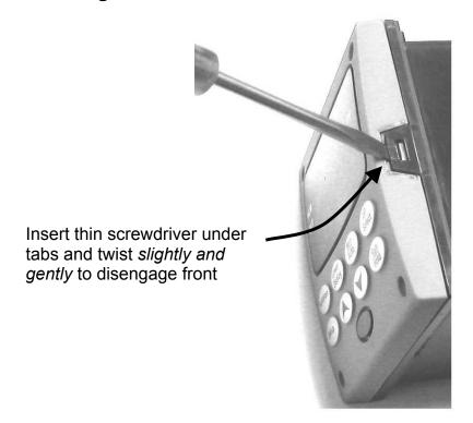
Using a thin screwdriver, *gently* twist the screwdriver to pry the side tabs from the front face. Pry just enough to release it, *otherwise you'll bend or break the tab*. If you break or bend the tab and can't reattach the front snugly, you'll need to reattach the front using the 4 NEMA4 screws provided. See Figure 2-3 on page 15.
