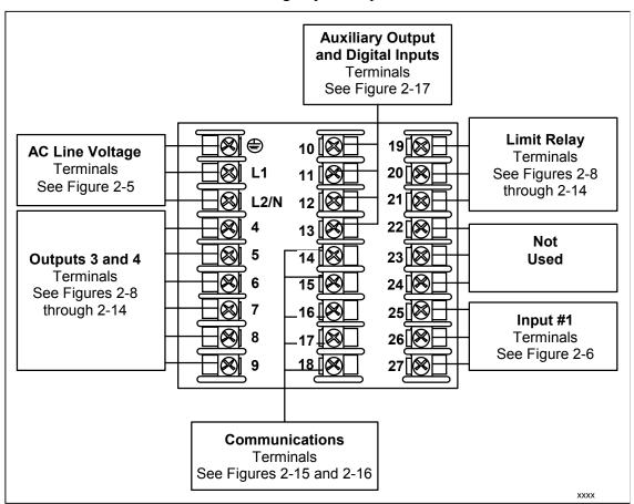
Figure 2-4 Composite Wiring Diagram
