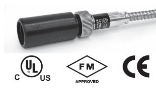
This sensor features a high temperature and high sensitivity ultraviolet (UV) tube for monitoring gas or oil flames which cycle on and off frequently. The Eclipse flame safeguard checks for a short-circuited, or "runaway" scanner at the beginning and end of each flame cycle.
