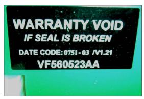
Some early units with the date code **0748-03 through 0801-03** may not be stamped on the front. If the label on the back of the unit shows -03 after the 4-digit date code, you can mark the 03 on the bottom front with a permanent marker to help with future identification.
