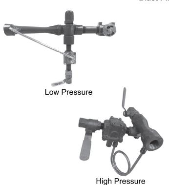
Eclipse Blast Pilot Mixers utilize low pressure gas (6" w.c. to 15" w.c.) and air from a low pressure blower (4 oz. to 32 oz.) and can be used on open or sealed burner applications.
