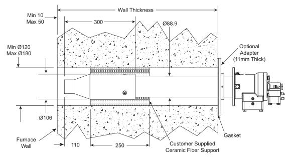
Make sure the gasket is installed between the mounting flange and the chamber wall. Locate the end of the ceramic combustor between 10mm and 50mm inside furnace wall. Clearance hole in the chamber wall must be between 120mm and 180mm in diameter. Pack the gap with ceramic fiber as stated above to the dimensions shown.
