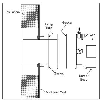
Figure 3.1. Mounting with Access to Inside of Appliance
