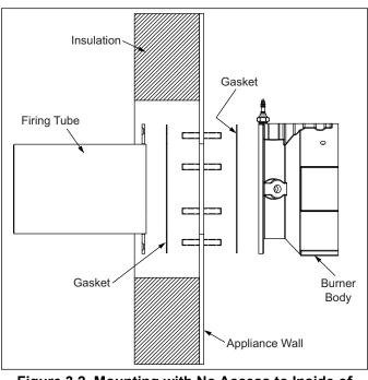
Figure 3.2. Mounting with No Access to Inside of Appliance
