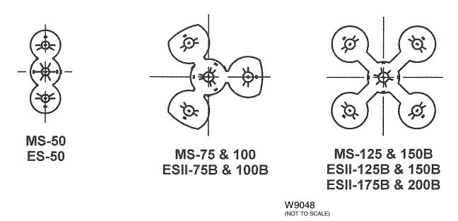
Figure 21. LP Nozzle Orientation
