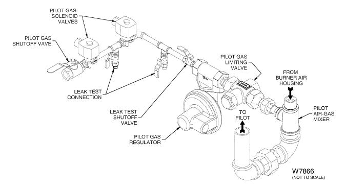
Figure 24. Pilot Manifold Detail
