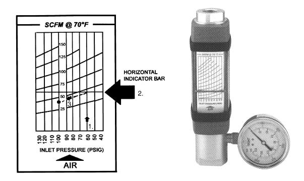
Figure 18. Compressed Air Flow Meter and Scale
