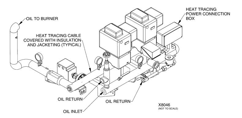
Figure 13. Heavy Oil Manifold Heat Tracing Kit
