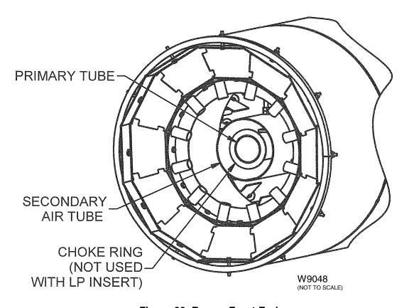
Figure 22. Burner Front End
