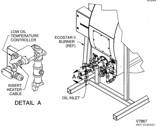
Figure 14. Heavy Oil Insert Heater
