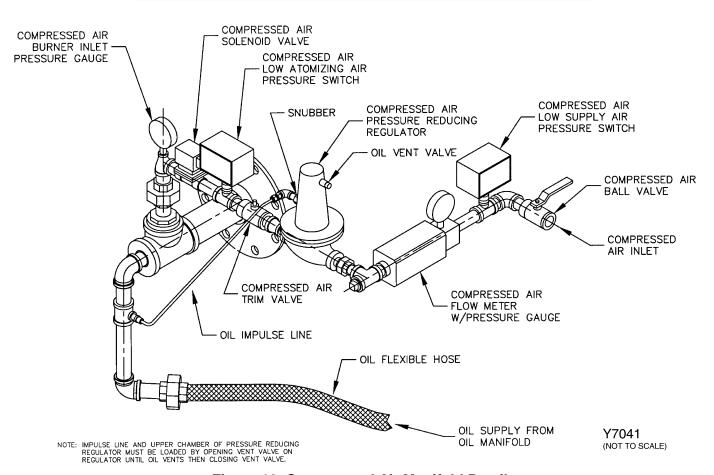
Figure 16. Compressed Air Manifold Detail
