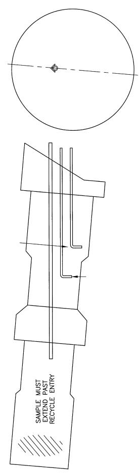
WELD 1/2" [DN 15] SAMPLE PIPE DIRECTLY ABOVE ASPHALT INJECTION USING 2 — 4" [51 — 102MM] STANDOFFS. EXTEND END OF PIPE 18 — 24" [460 — 610MM] PAST ASPHALT INJECTION, LEAVE APPROXIMATELY 12" [305MM] OF PIPE EXPOSED TO OUTSIDE. BOTH ENDS OF PIPE SHOULD BE THREADED, END INSIDE OF DRYER SHOULD HAVE A 90° ELBOW POINTING DOWN. OUTSIDE END CAN BE CAPPED WHEN NOT IN USE. ANGLE WELDED TO SAMPLE PIPE FROM ASPHALT INJECTION TO 4" [102MM] PAST ELBOW WILL PREVENT WEAR.
