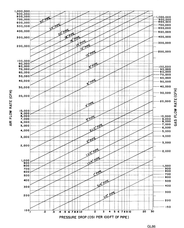
Figure 9. Simplified Gas and Air Flow Chart (@ Atmospheric Conditions)
