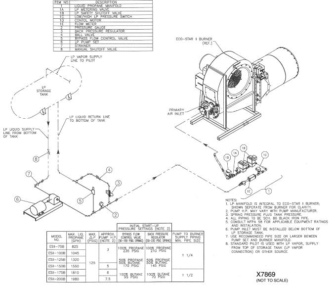
Figure 19. Typical Schematic of LP Piping
