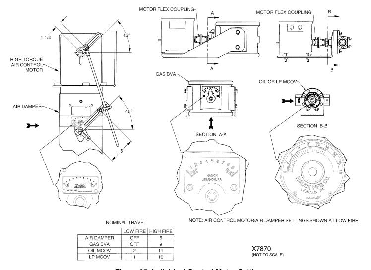
Figure 25. Individual Control Motor Settings
