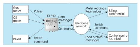
DL240 data collection device including remote-controlled digital output to switch from gas to oil
