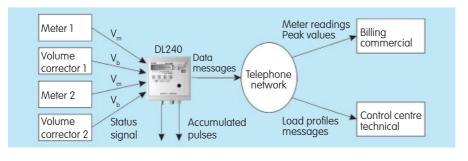
DL240 data collection device for a dual-stream gas metering system
