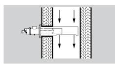
At flow velocities of > 15 m/s, the protective flame tube FPT is used to protect the flame from being cooled.
