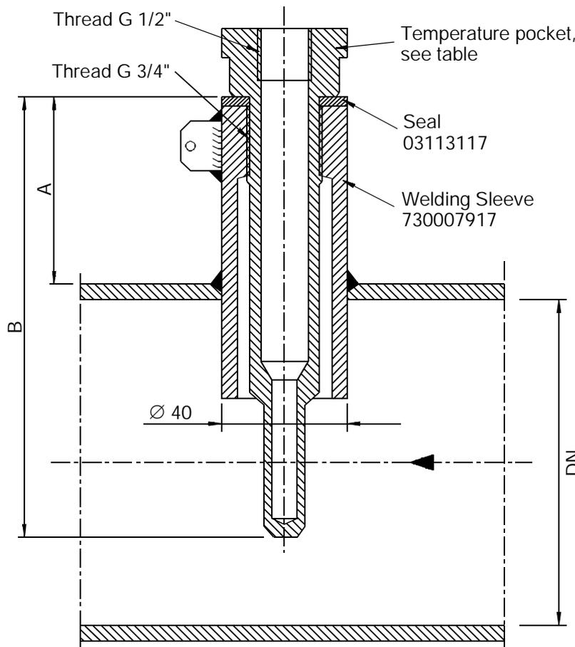
The pocket is suitable for Pt100 temperature probes with an installation length (EBL) of 160 mm. It consists of the temperature pocket, the seal and the welding sleeve (article number for the complete pocket: 73012100). The welding sleeve is suitable for a pipe diameter from DN 80 upwards.
