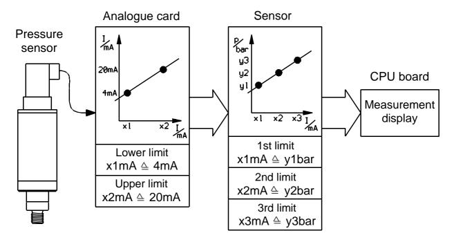
Figure: Correction of the pressure sensor characteristic.
