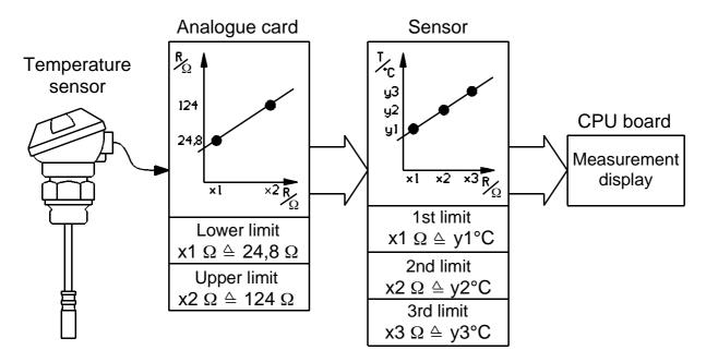
Figure: Correction of the temperature sensor characteristic.
