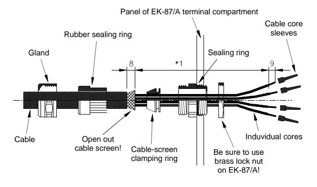
Connection of the cable screens to the PG cable glands:
