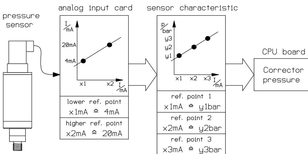
Fig. 3.4.6-10: Correction of the pressure sensor characteristic
