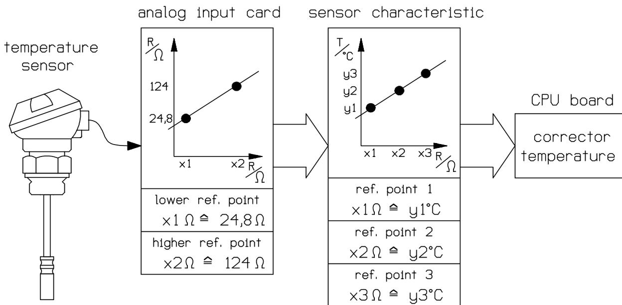
Fig. 3.4.6-22: Correction of the temperature sensor characteristic
