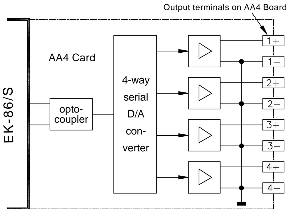
Fig. 4.2.3-1: Output assignment on the analogue output card
