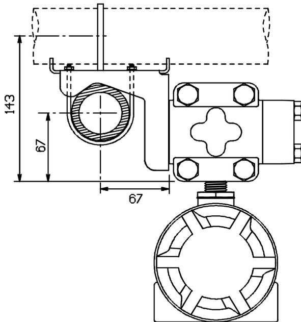
Mounting bracket for wall installation
