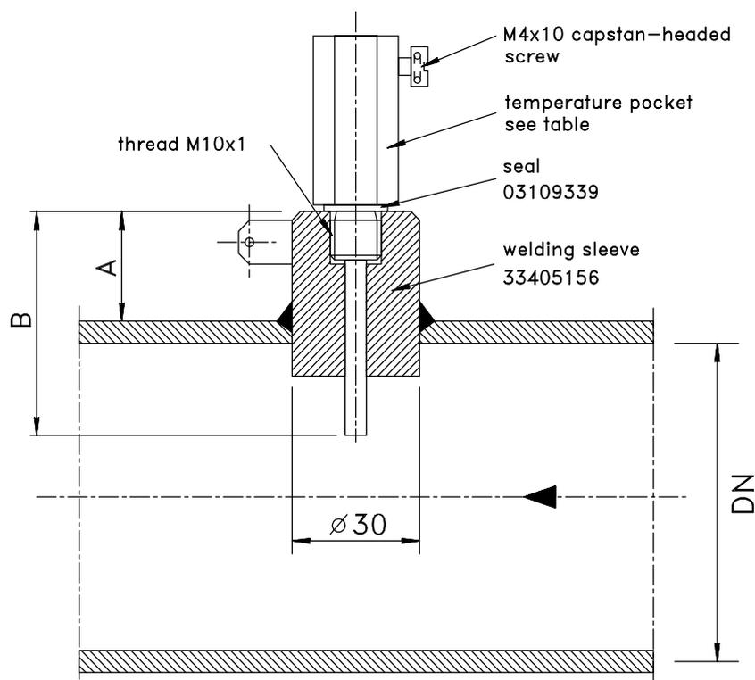
The pocket is suitable for PT100 temperature probes with an installation length of 50 mm. The complete pocket (article no.: 73012634) consists of the temperature pocket, the seal and the welding sleeve.
