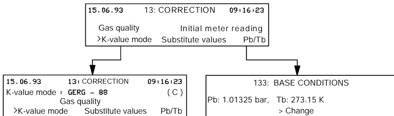
Fig. 3.1-2: Example: Correction menu
