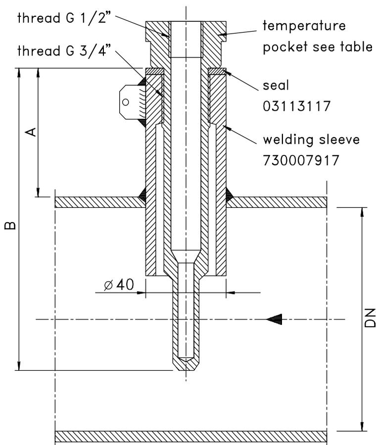
The pocket is suitable for PT100 temperature probes with an installation length (EBL) of 160 mm. It consists of the temperature pocket, the seal and the welding sleeve (article number for the complete pocket: 73012100). The welding sleeve is suitable for a pipe diameter from DN 80 upwards.
