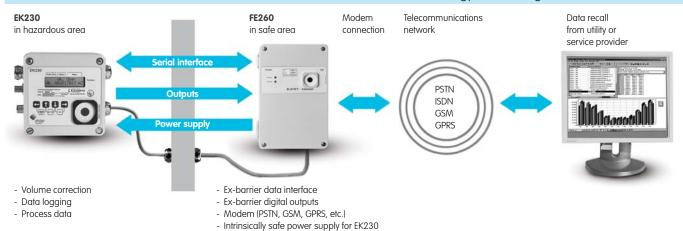
The Ex-barrier of the serial interface and the pulse outputs of the volume corrector are provided by the FE260 function extension unit. In addition, the intrinsically safe power supply of the volume corrector is guaranteed. The unit's modular concept allows the use of a modem for data communication or an interface for connection to other devices.
