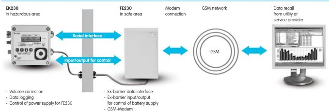
The FE230 function extension unit is a battery-operated GSM modem which allows data communication without exter-
