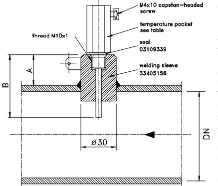
The pocket is suitable for PT100 temperature probes with an installation length of 50 mm. The complete pocket (article no.: 73012634) consists of the temperature pocket, the seal and the welding sleeve.
