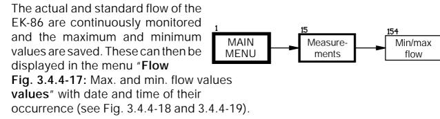
154: MAX. FLOW SINCE 17.06.93 15:29:57 Qnmax:021073.8 m3/h on 28.06.93 13:20:22 Qmax: 3673.9 m3/h on 24.06.93 16:41:21 >Qmax Qmin Delete
