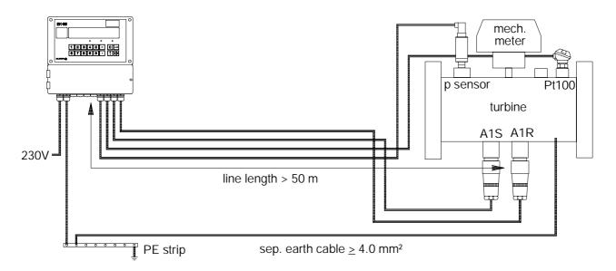
Fig. 2.2.1-1: Cable connection for cable lengths greater than 50 m
