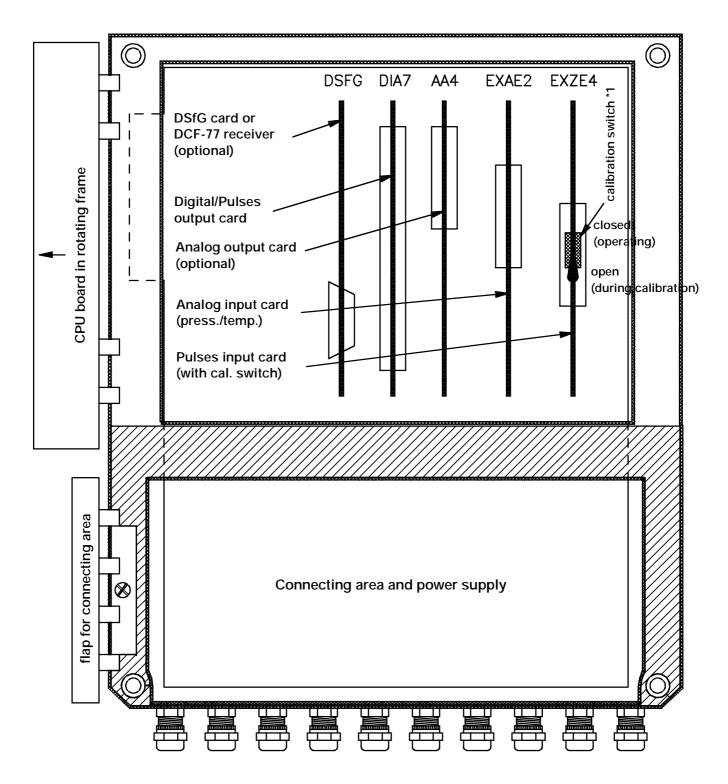
\*1) Calibration switch on the ExZe4 card only for the EK-86/W; with the EK-86/A it is on the front panel.
