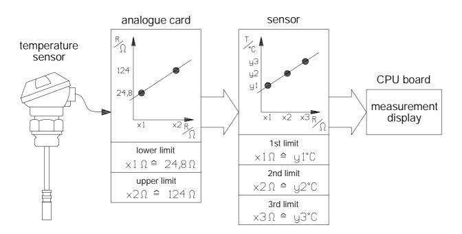
Fig. 3.4.2-1: Correction of the temperature sensor characteristic.
