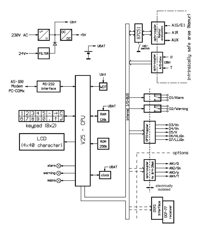
Fig. 1.2-1: Block diagram of EK-86/W and /A
