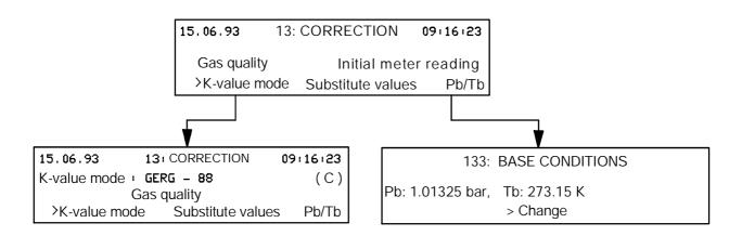
Fig. 3.1-2: Example: Correction menu
