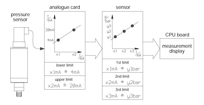
Fig. 3.4.1-1: Correction of the pressure sensor characteristic.
