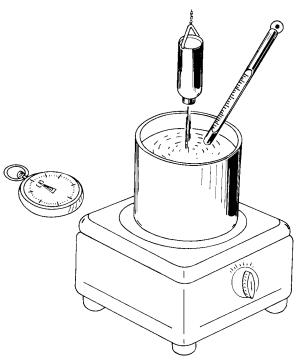
The Hauck Oil Viscometer is designed to provide an easy, convenient and inexpensive way of rapidly determining the temperature to which oil should be heated in order to arrive at the proper viscosity for atomization.
