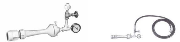
The Hauck "Ratio" Gas Torch combines a "Retain-A-Flame nozzle with an inspirator to produce a multipurpose torch designed for use where gas pressures from 10 to 30 psig are available. The inspirator assists in maintaining the roper air-gas ratio under all operating conditions. This torch is designed for rugged duty in open air applications.
