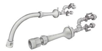
The Hauck "Booster" Torch combines a "Retain-A-Flame nozzle with a booster to produce a multipurpose torch designed for use where low pressure gas and compressed air (ranging from 30 to 120 psig) are available. The booster assists in maintaining the proper air-gas ratio under all operating conditions. This torch is designed for rugged duty in open air applications.
