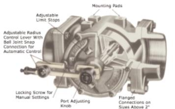
Valve flow rate is controlled by operating the lever to rotate the cylindrical piston for desired amount of port opening. The height of the rectangular port opening can be adjusted for the entire range of lever travel, by merely turning a single adjusting knob. This knob has *close* and *open* direction arrows, and a socket screw for positive position lockout.
