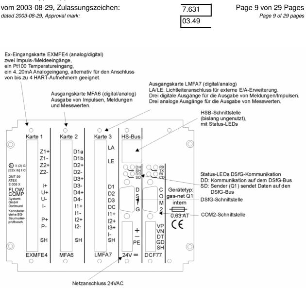
Figure 5: Rear view of the Q1 gas-net evaluation computer
