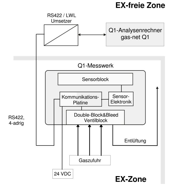
Figure 3: Schematic diagram of Q1 measuring unit and Q1 evaluation computer (gas-net
