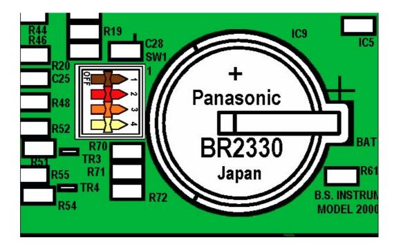
View of Microprocessor Board Showing Mode Switches and Backup Battery
