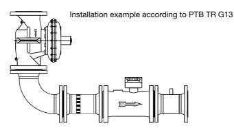
BLN 1 flow conditioner for installation in the inlet pipe and for use with high level perturbations
