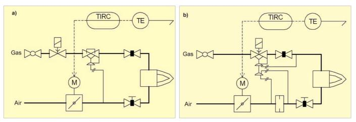
Fig. 5: Schematic diagram of pneumatic ratio control a) Air/gas ratio control, b) Variable air/gas ratio control
