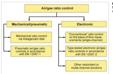
Fig. 2: Methods of ratio control individually for each specific system and should include MIN and MAX pressure switches for both gas and air (**Fig. 3**). Provided that the combustion chamber backpressure is not negligible compared to the air and gas supply pressures, the pressure switches must monitor the pressure differential to the combustion chamber.
