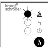
**1** Press the reset button during operation.
