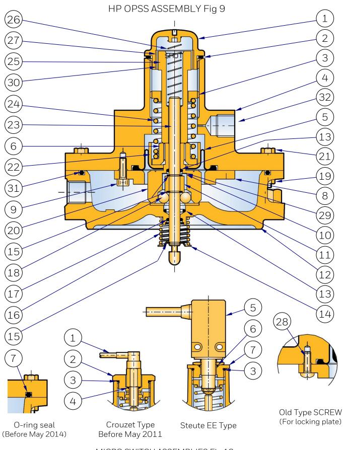
MICRO SWITCH ASSEMBLIES Fig 10 (For LP, MP & HP Assemblies)
