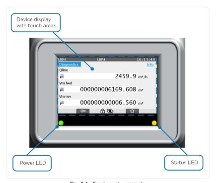
Fig. 6-1: Front panel – example
