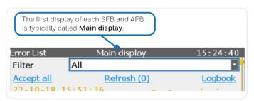
Fig. 6-3: The Main display ≙ 1<sup>st</sup> display of an AFB or SFB – example
