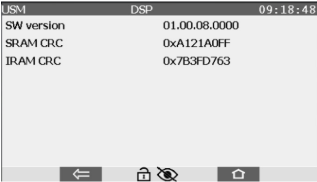
Fig. 8-2: Display DSP with checksums of its software components – example
