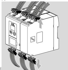
3 Disengage the BCU from the DIN rail.
