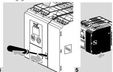
**6** Remove the old parameter chip card from the BCU and insert the new one.
