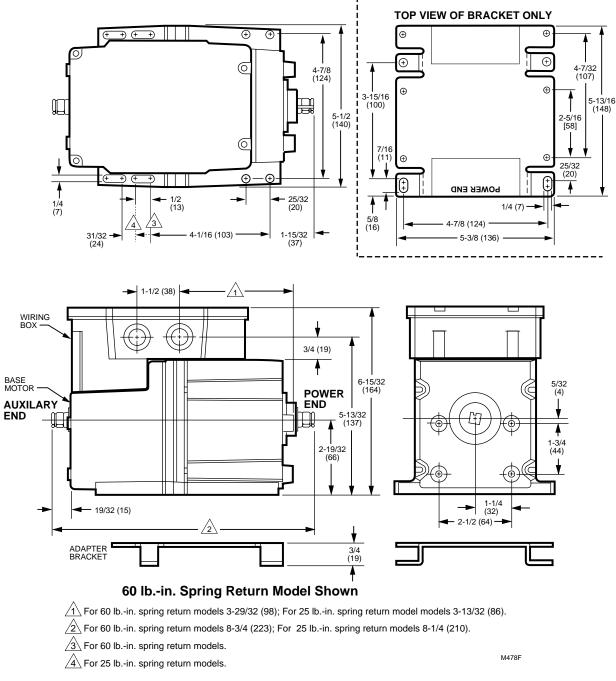
Fig. 1. M4185/M4186/M8175/M8185 mounting dimensions in in. (mm). NOTE: M4182/M8182 motors do not have auxiliary shaft, but all other dimensions are the same.
