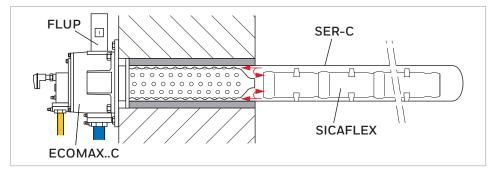
ECOMAX radiant tube heating
