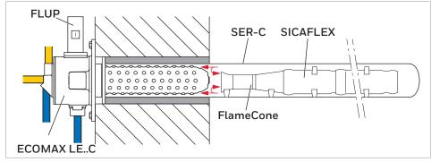
ECOMAX LE radiant tube heating
