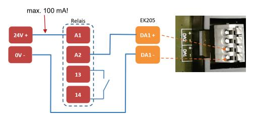
Most relays have an LED on the switch contact. If this flashes, you can assume that the output of the EK205 is correctly connected and functional.
