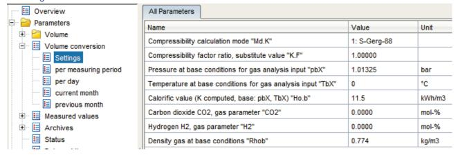
The possible inputs displayed will automatically adjust to the selected gas analysis method.
