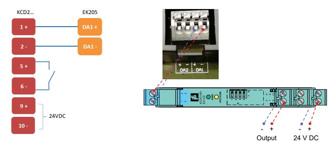
Most isolating amplifiers have an LED on each input. If this flashes, you can assume that the output of the EK205 is correctly connected and functional.
