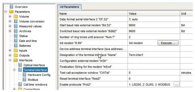
All the values listed in enSuite under "Parameters" can be found in the "Serv." and "Admin" display tabs of the EK205 using the same path.
