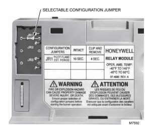
Fig. 13. Selectable site-configurable jumpers.
