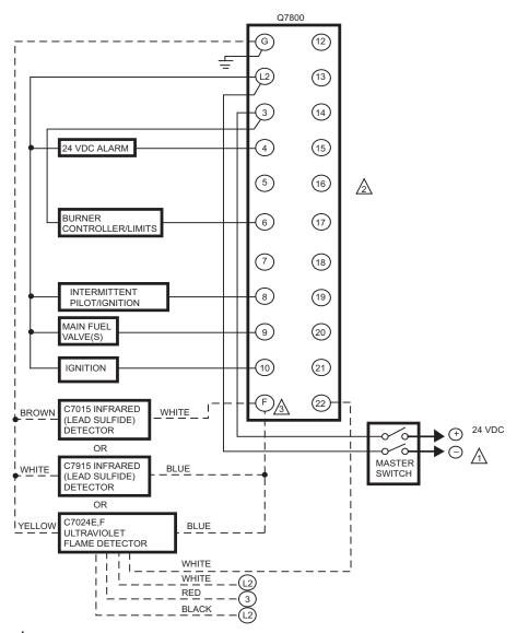
⚠ 24 VDC POWER SUPPLY. PROVIDE DISCONNECT MEANS AND OVERLOAD PROTECTION AS REQUIRED.
