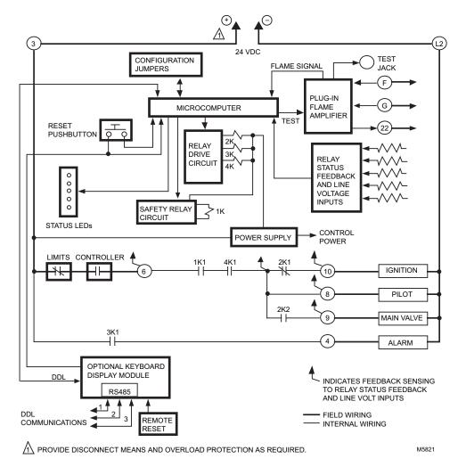
Fig. 4. Internal block diagram of the RM7824A (see Fig. 8 for detailed wiring instructions).
