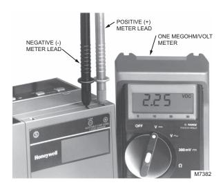
Fig. 14. Flame signal measurement.
