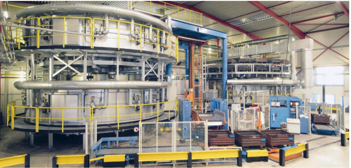
Annealing furnace, IOB works photograph
