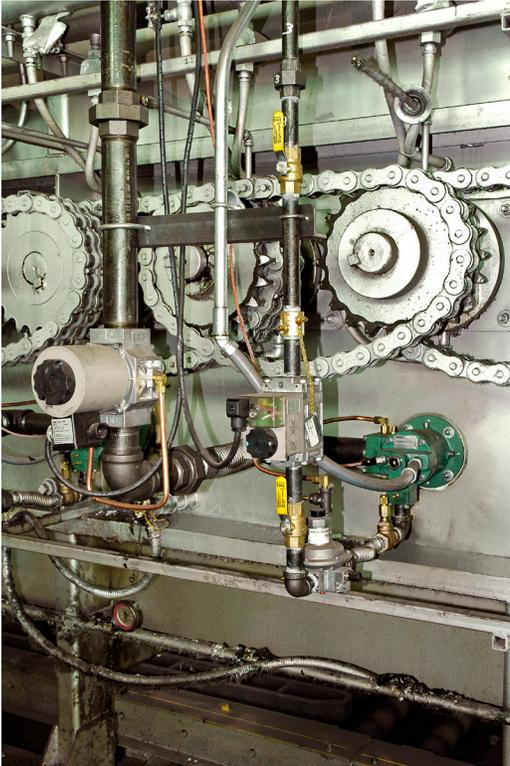
*TJ Burner set up for high/low pulse firing*
