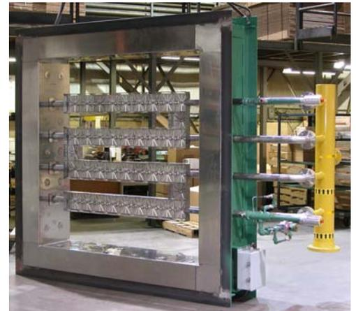
Packaged FlueFire Burner prior to installation
